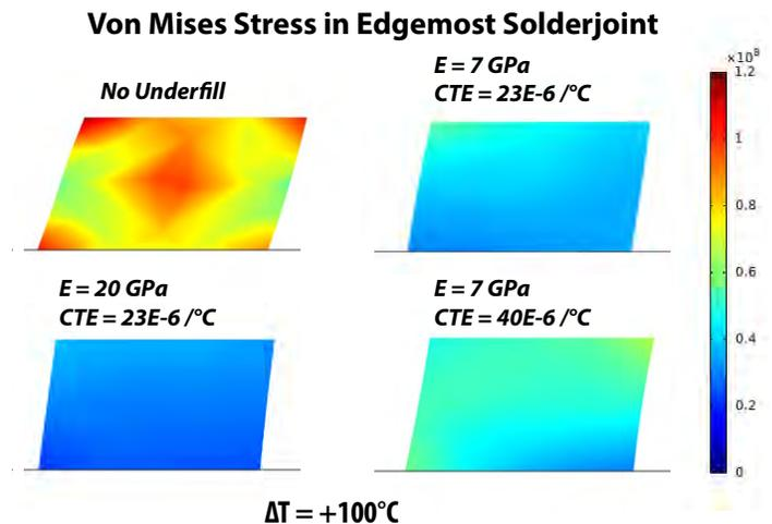
Figure 36: Von Mises (peak shear stress) in the edge-most solder bar under a temperature cycle change of  $\Delta T = +100^\circ\text{C}$ . Four different underfill conditions are simulated, with changing Youngs modulus ( $E$ ) of the underfill, and different CTE as well. Note that mechanical deformation has been exaggerated by 20x in all cases.
