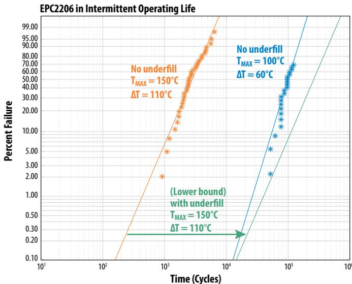
Note: The parts with underfill (Namics U8437-2) are still under test with no failures after 53k cycles so the green Weibull "fit" represents a lower bound
