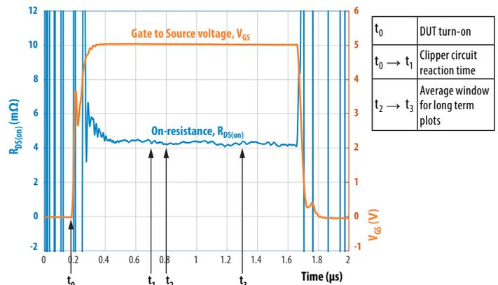
Figure 13: High time resolution oscilloscope waveform of the  $R_{DS(on)}$  in the first 1–2  $\mu\text{s}$  after a switch on transition. This waveform was taken on an EPC2218 after 1000 hours of continuous resistive hard-switching. Note that there is no evidence of the “fast dynamic  $R_{DS(on)}$ ” recovery seen in other GaN technologies.
