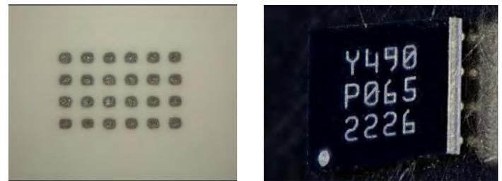
Figure 31: (Left) Solder stencil pattern squeegeed onto ceramic substrate. (Right) DUT3 after reflow onto substrate.
