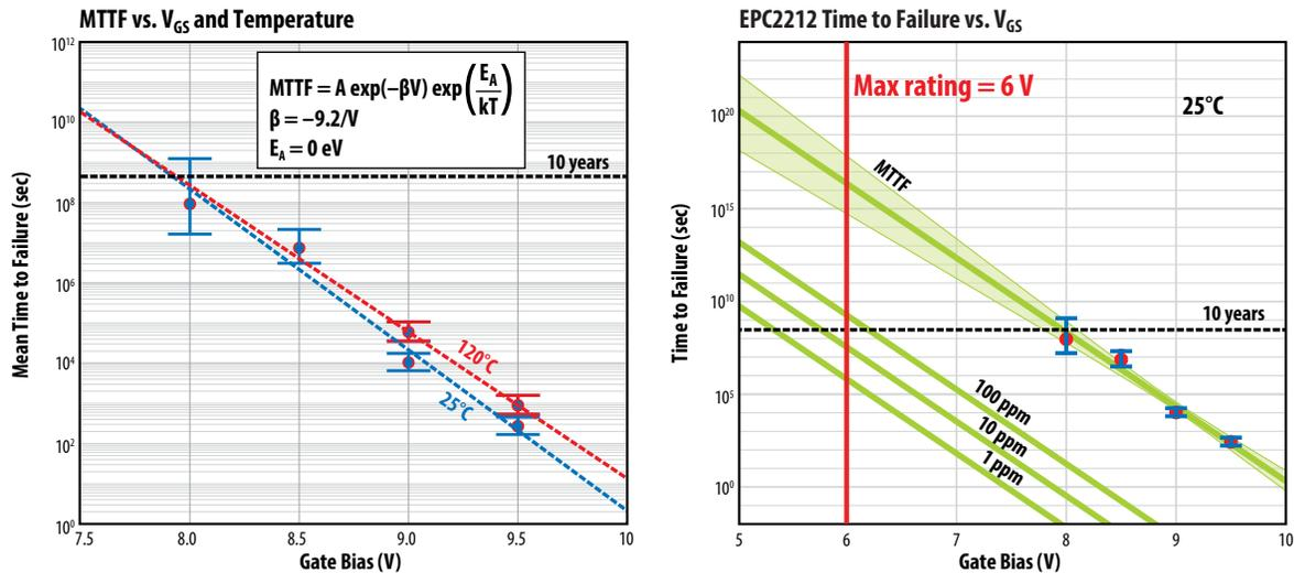
Figure 2: On the left is the mean time to failure (MTTF) for EPC2212 eGaN FETs versus V<sub>GS</sub> at both 25°C and 120°C. On the right is a graph that shows the various probabilities of failure versus V<sub>GS</sub> at 25°C.
