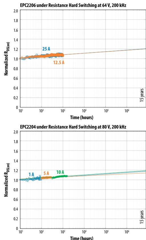
Figure 15: Effect of switch current on dynamic  $R_{DS(on)}$ . (top) Two EPC2206 devices were tested under resistive hard switching at 64 V, 200 kHz. (bottom) The same device was tested under inductive hard switching and three different currents at 80 V, 200 kHz. No discernible difference was found in the slope or intercept of the log(t) growth characteristics.
