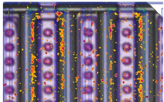
Figure 8: A magnified image of an EPC2212 eGaN FET showing light emission in the 1–2  $\mu\text{m}$  wavelength range (SWIR) that is consistent with hot electrons. The SWIR emission (red-orange) has been overlaid on a regular (visible wavelength) microscope image.
