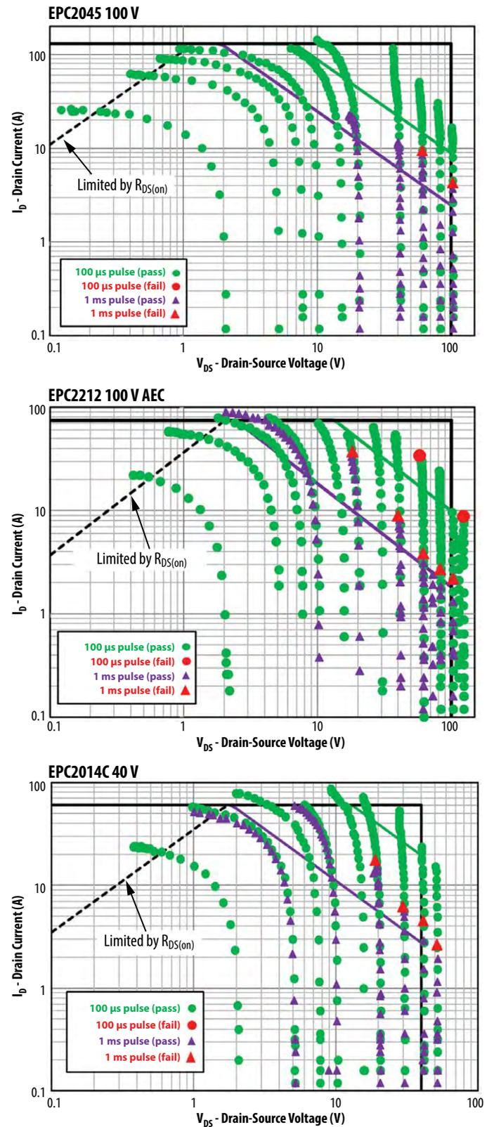
Figure 20: SOA results for EPC2045, EPC2212, EPC2014C. Measurements for 1 ms (purple triangles) and 100 μs (green dots) pulses are shown together. Failures are denoted by red triangles (1 ms) or red dot (100 μs). Note that for all parts, all failures occur outside the data sheet SOA region.
