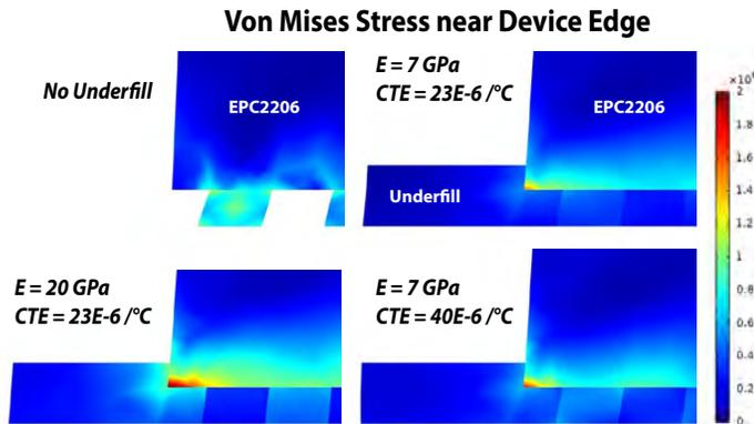
Figure 37: Von Mises (peak shear stress) in the edge-most solder bar under a temperature cycle change of  $\Delta T = +100\text{C}$ . Four different underfill conditions are simulated, with changing Young's modulus ( $E$ ) of the underfill and different CTE as well. Note that deformation has been exaggerated by the same scale in each picture.
