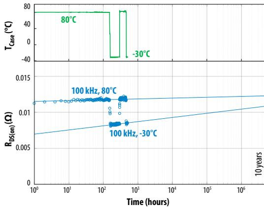
Figure 16: Effect of alternating hot-cold conditions on dynamic  $R_{\text{DS(on)}}$  for an EPC2059. (Top) Case temperature versus Time, as controlled by a thermoelectric cooler. (Bottom)  $R_{\text{DS(on)}}$  versus Time. Switching is continuous throughout at 100 V and 100 kHz.
