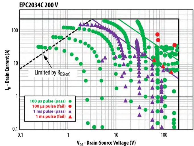
Figure 19: EPC2034C SOA plot. The "Limited by  $R_{DS(on)}$ " line is based on data sheet maximum specification for  $R_{DS(on)}$  at 150°C. Measurements for 1 ms (purple triangles) and 100  $\mu$ s (green dots) pulses are shown together. Failures are denoted by red triangles (1 ms) or red dot (100  $\mu$ s). Note that all failures occur outside the data sheet SOA region.
