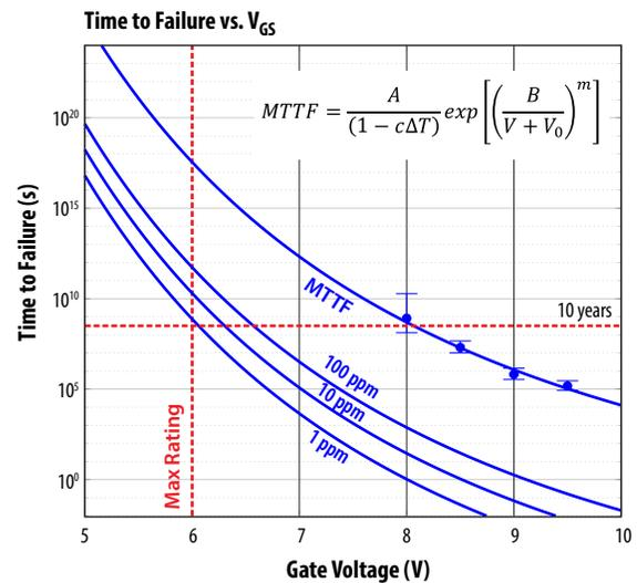
Figure 4: EPC2212 MTTF vs.  $V_{GS}$  at 25°C MTTF (and error bars) are shown for four different voltage legs. The solid line corresponds to the impact ionization lifetime model. Extrapolations of time to failure for 100 ppm, 10 ppm, and 1 ppm are shown as well.
