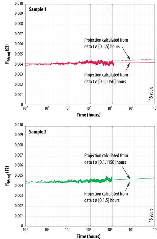
Figure 12: Comparison of  $\log(\text{time})$  fits to the  $R_{DS(on)}$  data, where the dashed line represents the fit over the first 5 hours, while the solid line represent the fit over the full 1150 hours. Data for two samples of EPC2218 are shown. Note that the short-term fit has a similar projection to the long-term fit, with small random differences of  $\pm 10\%$  on the 15 year projection.
