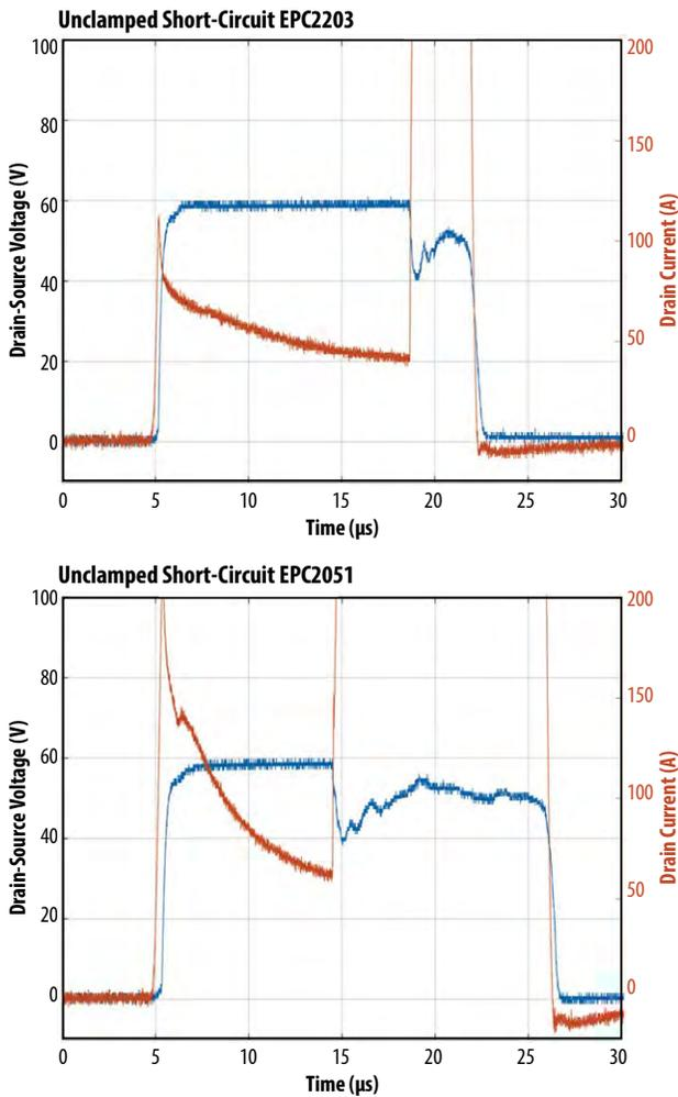
Figure 22: Fault under load test waveforms for a typical EPC2203 (top) and EPC2051 (bottom) at  $V_{DS} = 60\text{ V}$ ,  $V_{GS} = 6\text{ V}$  and a  $25\ \mu\text{s}$  drain pulse. The abrupt rise in drain current marks the time of catastrophic thermal failure.
