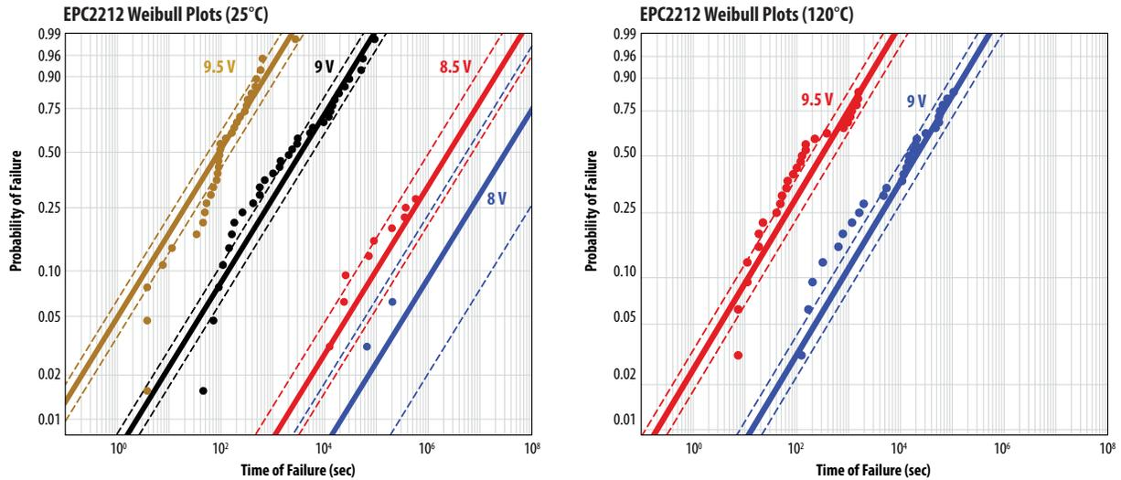
Figure 1: Weibull plots of gate-to-source failures of EPC2212. Note that very few failures occur even at 8 V<sub>GS</sub>, yet the device has a maximum V<sub>GS</sub> rating of 6 V. The data on the top is at 25°C and the data on the bottom is at 120°C.
