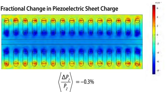
Figure 30: Fractional change in piezoelectric sheet charge for an EPC2206 under strain from 4 mm board deflection. The area averaged change in piezoelectric charge is less than -0.3%, while the peak change is around 0.8% in the immediate vicinity of solder bars. These changes in piezoelectric polarization are too small to create observable changes in device parameters  $V_{TH}$  or  $R_{DS(on)}$ .
