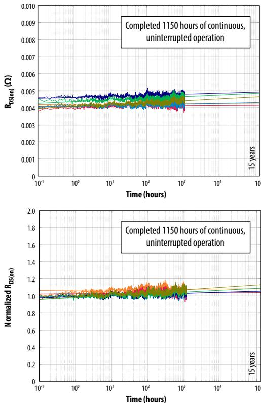
Figure 11: Long-term dynamic  $R_{DS(on)}$  for six samples of EPC2218 eGaN FETs under continuous resistive hard-switching operation for over 1000 hours at ambient temperature and a bias of 100 V. The graph on the top shows  $R_{DS(on)}$  versus Time, while the bottom graph shows  $R_{DS(on)}$  normalized to its value after the first 10 minutes. Note that even over 1000 hours of operation,  $R_{DS(on)}$  does not deviate from a simple  $\log(\text{time})$  growth dependence.
