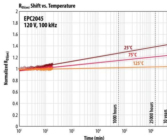
Figure 10: The  $R_{DS(on)}$  of a fifth-generation EPC2045 eGaN FET over time at various voltage stress levels and temperatures. On the left, the devices were tested at 25°C at voltages from 60 V to 120 V. The graph on the right shows the evolution of  $R_{DS(on)}$  at 120 V at various temperatures.
